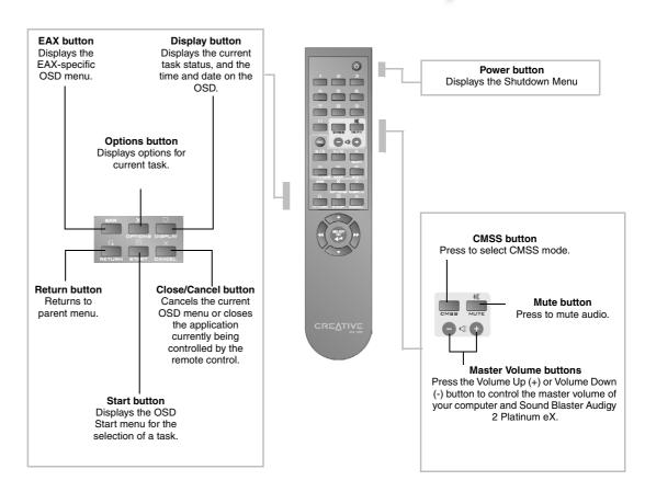
Figure 1-5: Other Buttons on the Remote Control.
